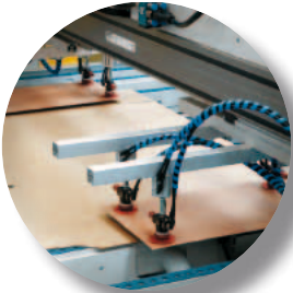
Linear motor driven placing unit of a folding & glueing machine
